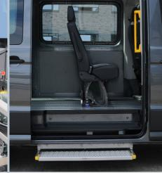
Step and grab handle at the side entry allow easy access to the passenger compartment.
