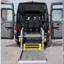
Wheelchair safely enters the vehicle via the lift.
